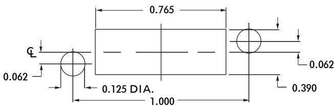
RECOMMENDED CHASSIS CUT-OUT
