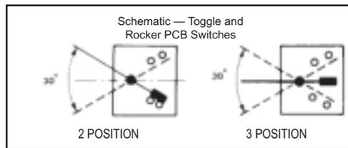
**CAUTION — MANUAL SWITCHES ARE AFFECTED BY HEAT, CLEANING SOLVENTS AND FLUX. EXTREME CARE SHOULD BE EXERCISED DURING HAND SOLDERING AND WAVE SOLDERING TO PREVENT SWITCH CONTAMINATION.**
