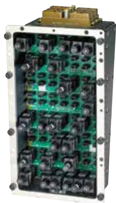
56 CB military helicopter panel (PCB + casing)
