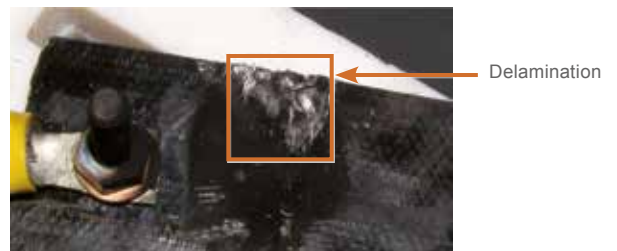
230 VAC Fault without arc fault protection: delamination of the fibers
