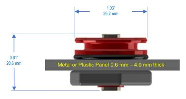
For complete dimensions, download 3D Step files of Terminal and Accessories at Rebling.com
